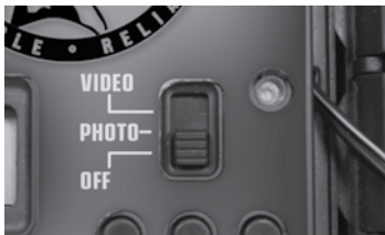
Slide Switch To Desired Setting The Camera Will Automatically Enter Active Standby Mode After 15 Seconds!
